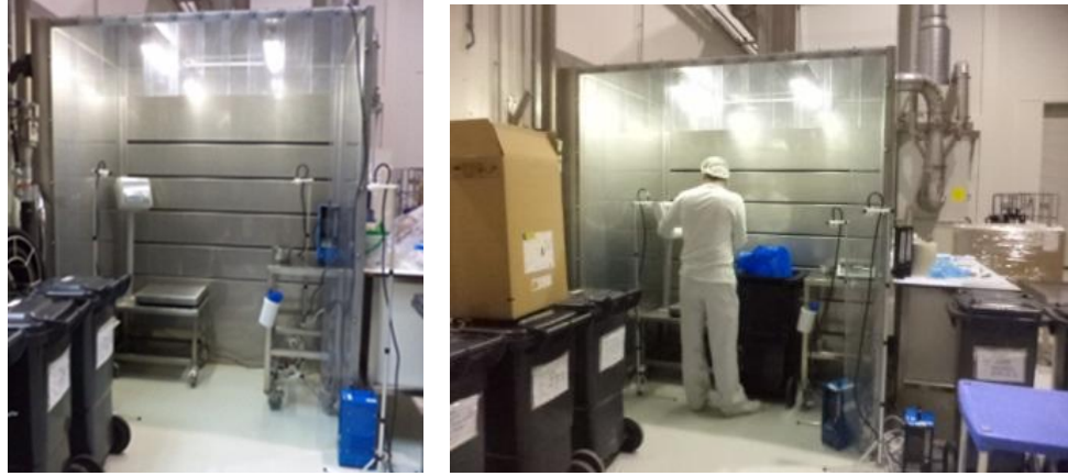
Figure 10: Work practices in a back flow booth
