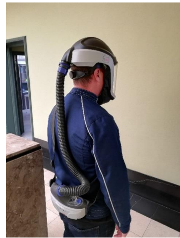
Figure 15: Powered Air Purifying Respirator (PAPR), (courtesy: IFF)
