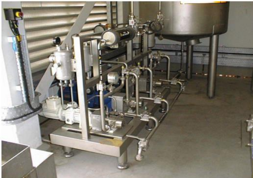
Figure 9: Example of Enzyme Transfer Pump Sets (source: AISE Guidelines for the Safe Handling of Enzymes in the Detergent Manufacturing).
