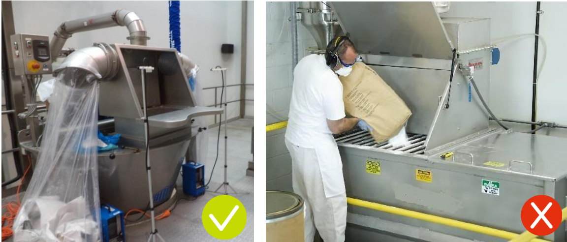
Figure 12: Examples of dumping stations. Powdered enzymes might be an issue in the right picture, especially if proteases are handled (uncovered arms)
